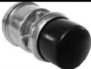
SSW2814 Push Button Switch PIC 9900-9014; 2-Screw Terminals ON-OFF (Normally OFF) Switch 2 Threaded Bosses with Screws for Wire Connections Plastic Buffer O-Ring Seal in Mounting Stem Protective Cap and Face Nut Assembly REPL.: DELCO 0907
